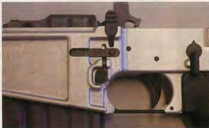
A new feature found on the XM110 is KAC's ambidextrous magazine release, seen here on a prototype receiver in the white.
